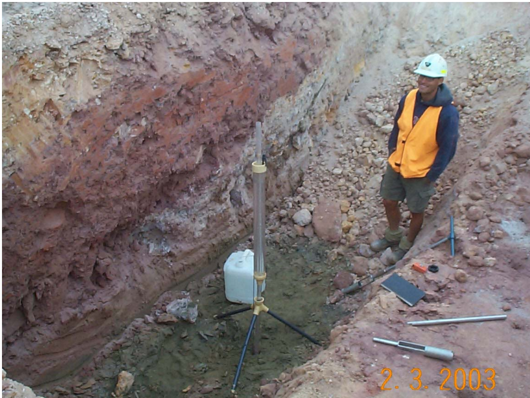
Figure 2.4 Field hydraulic conductivity testing.
